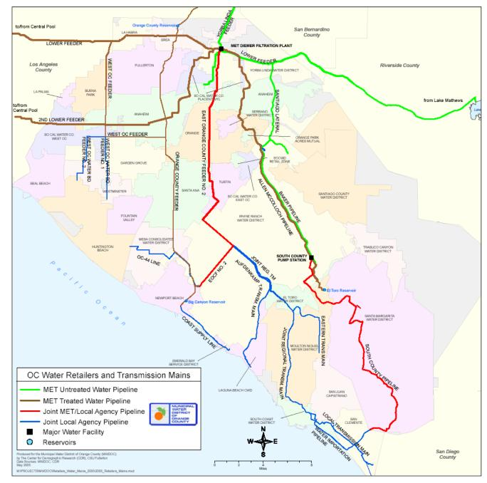
**Figure 2. MWD Feeders and Transmission Mains**
